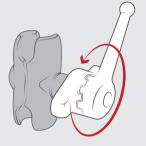
This wrench provides the extra leverage needed to tighten the mount in cold weather or in small spaces
