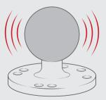
Rubber ball provides vibration damping
