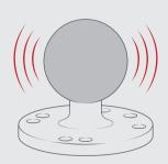
Rubber ball provides vibration damping
