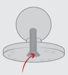
Steel bolt reinforces the post to provide maximum support even in rough environments
